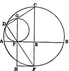
produce them to meet the O ABC in C and F; then CF is the diameter of the  $\odot$  ABC, and is || to PG(2);  $\therefore$  CF is  $\bot$  to AB; hence it bisects AB in E (iii.). Through F draw FH || to AB, and produce GP to meet it in H.
